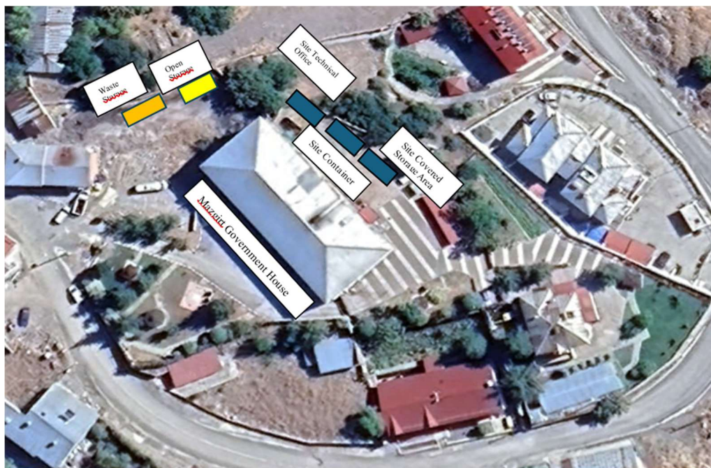
Figure 4 - Tunceli Mazgirt Government House Building Temporary Storage and Container Areas
