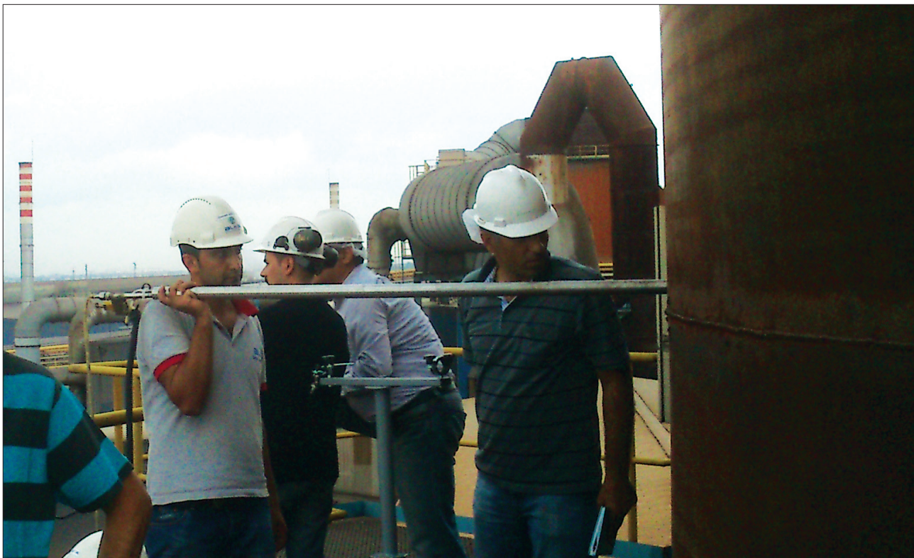
Picture 8 – Measurement of the emission from the chimney of an iron-steel facility during an environmental inspection.
