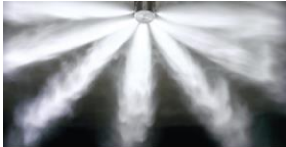
Figure 5. Discharging Novec 1230 from the system
