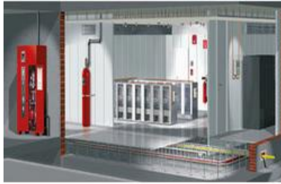
Figure 4. Examples of total flooding systems where Novec 1230™ is used
