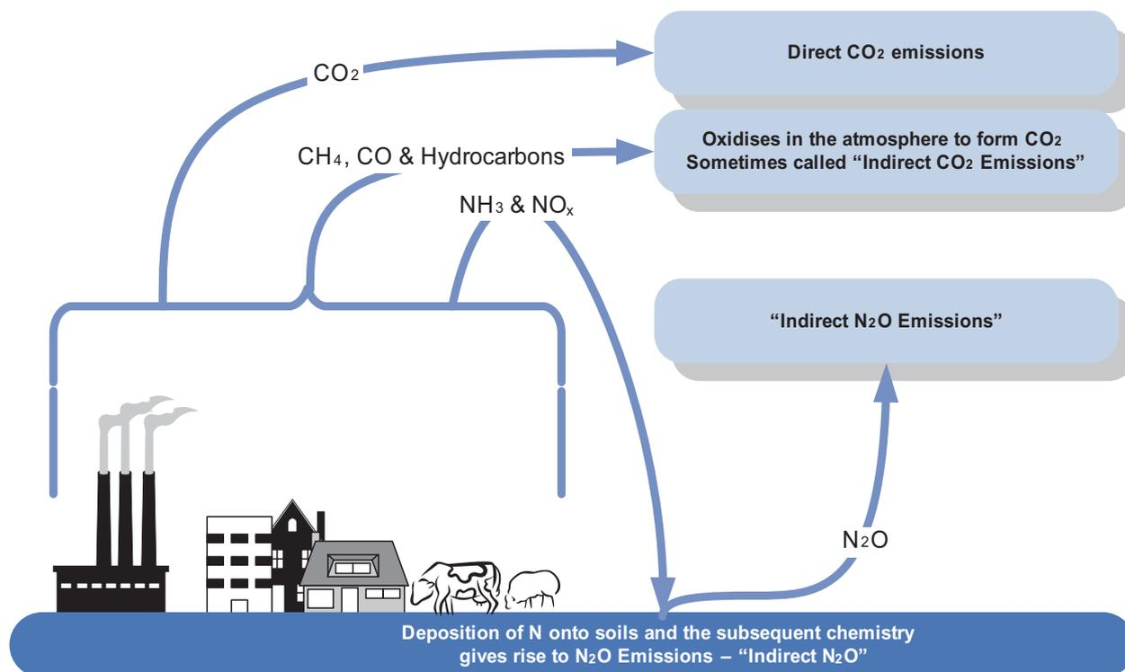
Figure 5 - Direct CO<sub>2</sub> and Indirect N<sub>2</sub>O
