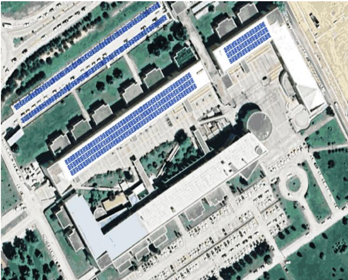
Figure 8 Sakarya Government Office Roof Top PV Layout Plan
