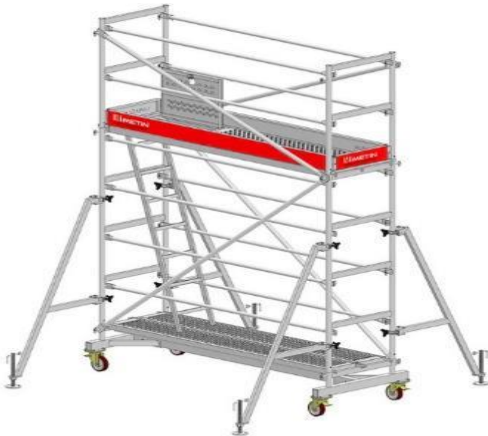
Figure 12 Mobile Scaffolding Sample Demonstration
