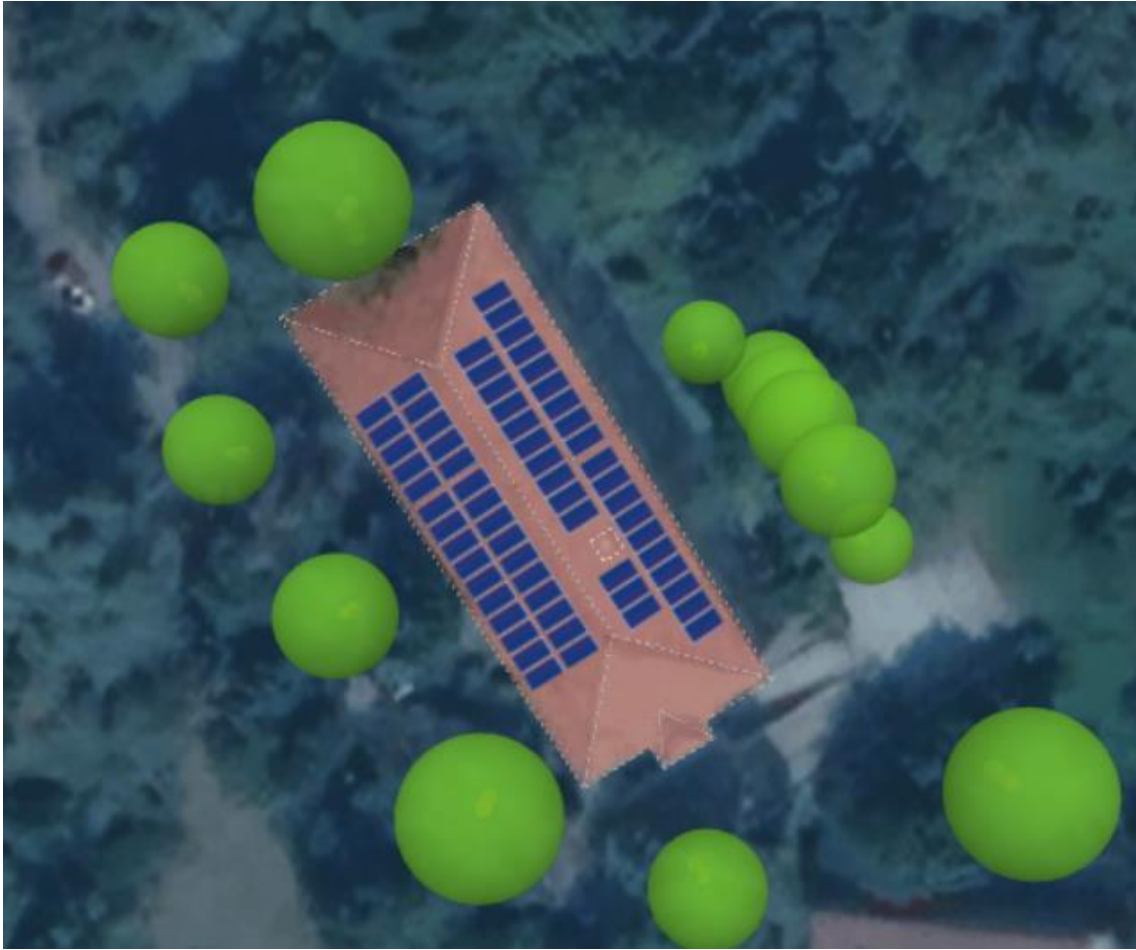
Figure 9 BOĞAZIÇI UNIVERSITY KANDİLLİ CAMPUS NEW GEOPHYSICS BUILDING Roof Top PV Layout Plan
