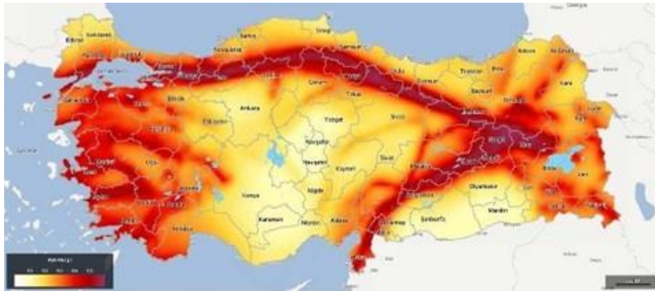
Figure 1. Probabilistic Seismic Hazard Map of Turkey 6 (SA at 0.2s – 475 yrs -10 percent in 50 yrs), AFAD
