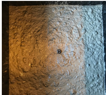
RFID tag in concrete cube
