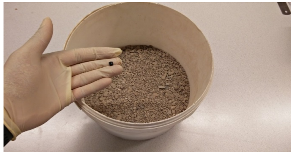
RFID tag in aggregate
