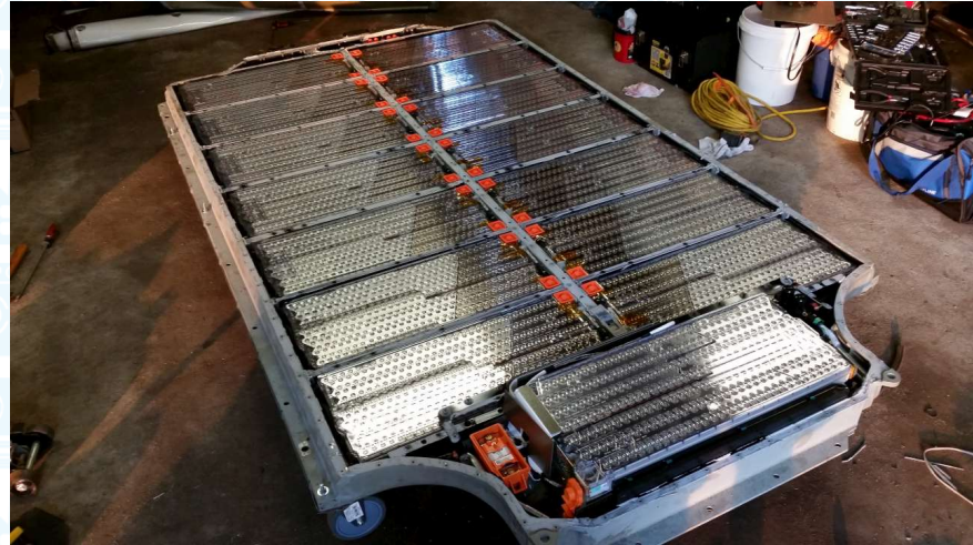
Battery pack of a Tesla model 3
